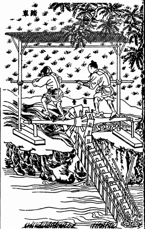
Managing the supply of water in pre-industrial China: this two-man chain pump was known as the 'dragon's backbone'. ILLUSTRATION FROM THE TIEN-KUNG K'AI-WU COLLECTION (17th century).
